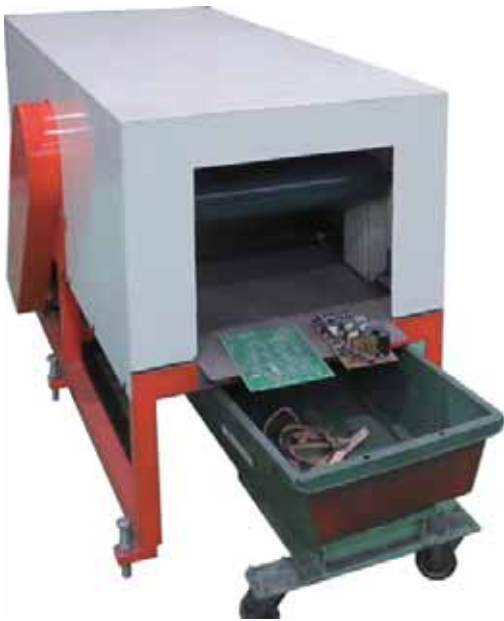
KBHS600 (single-side peeling type) (W: 970 mm, L: 2,000 mm, H: 1,115 mm)
